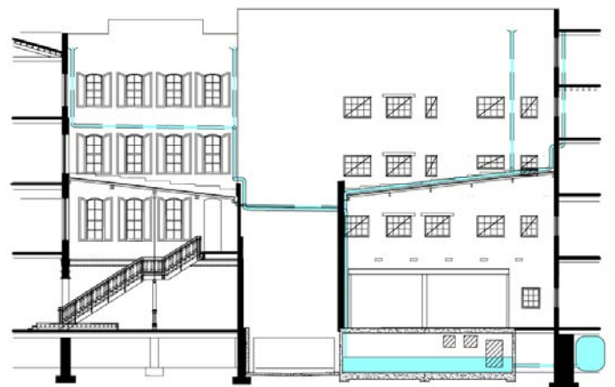
Detail of the Rainwater Catchment System
